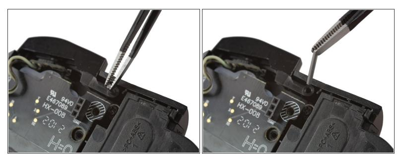
• Use a pair of tweezers to remove the metal pin which holds the bumper in its place.
