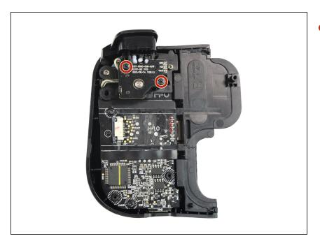
Use a Phillips #0 screwdriver to remove the two 4.4 mm-long screws securing the trigger board.
