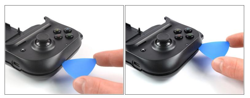
• Slide the opening pick along the right edge to loosen the plastic clips.
