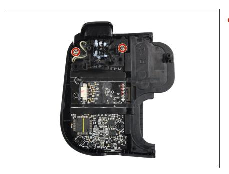
Use a Phillips #0 screwdriver to remove the two 7.0 mm-long screws securing the trigger.
