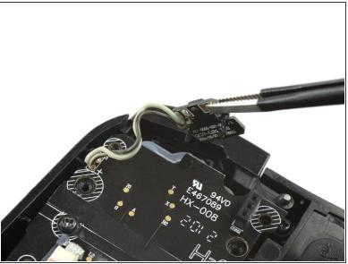
Use a pair of blunt nose tweezers to lift out the shoulder button board.
