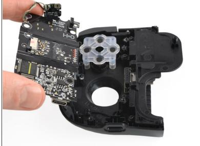
Pull the mainboard straight out of the frame to remove it.
