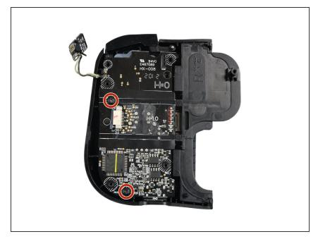
Use a Phillips #0 screwdriver to remove the two 5.9 mm-long screws.
