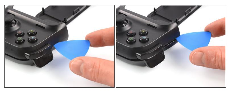
Slide the opening pick along the top edge to loosen the remaining plastic clips.
