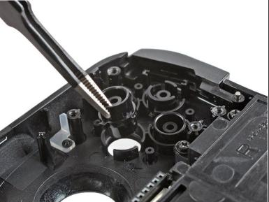
• Use a pair of tweezers to remove the face buttons.
