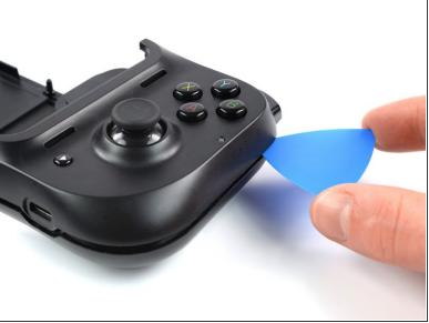
Slide the opening pick along the right edge to loosen the plastic clips.
