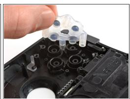
Remove the rubber cover by pulling it upwards.
