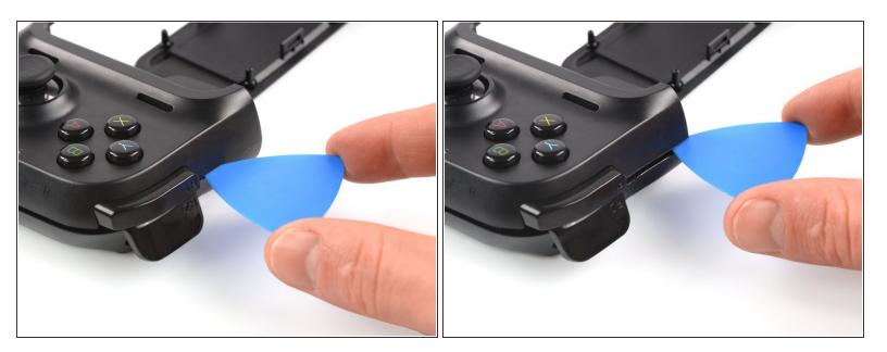
Slide the opening pick along the top edge to loosen the remaining plastic clips.
