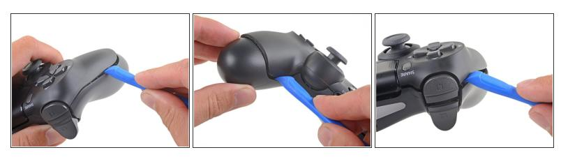
Use the opening tool to separate the panels by releasing the plastic clips around the perimeter of the controller.
