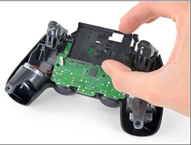
Remove the battery bracket.
