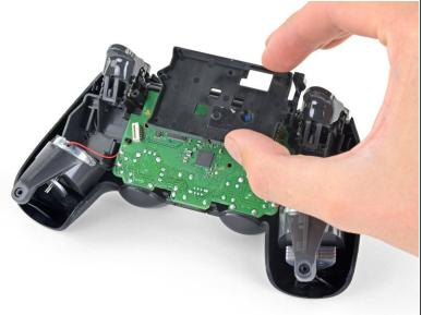
Remove the battery bracket.
