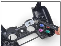
Use your fingers or a pair of <u>tweezers</u> to remove the three silicone conductive rubber pads from the controller buttons.
