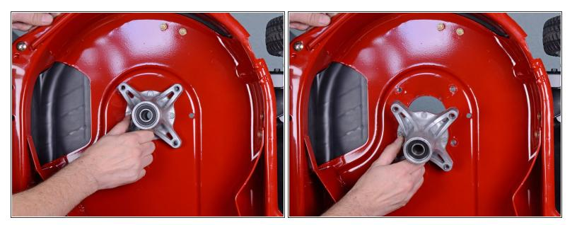
Remove the spindle.
