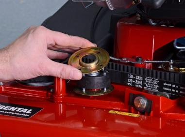
Remove the upper belt guide from the pulley.
