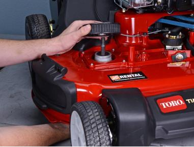
• While holding the spindle shaft from underneath, lift the sprocket up to remove it.
