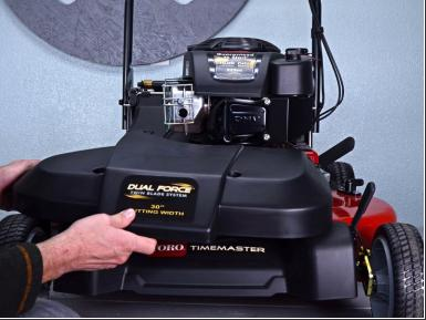
Pull the belt guard straight off the front of the mower to remove it.
