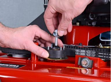
Remove the pulley bolt and washer.
