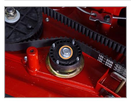
Use a 1/2 inch socket to remove the left pulley bolt
