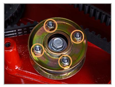
Use a 3/8 inch socket to remove the four bolts securing the upper belt guide to the pulley.
