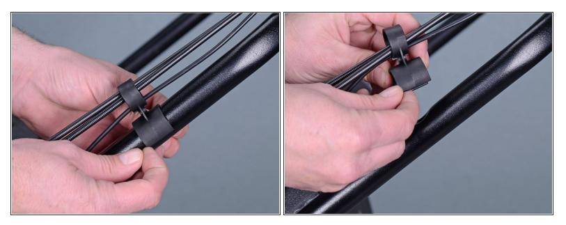
• Use your fingers and press up from the bottom to remove the plastic cable guide from the handle.
