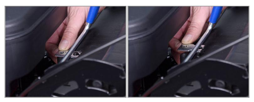
• Remove the cable guide plate.
