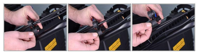
• Spread the cable guide apart and remove it from the cables.
