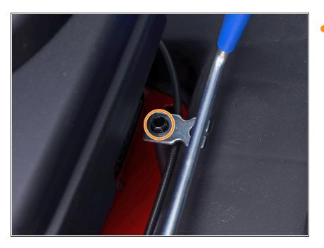
• Use a 3/8 inch socket to remove the cable guide plate screw.
