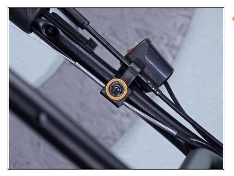
Use a 7/16 inch socket or wrench to remove the nut securing the kill switch and upper cable guide assembly.
