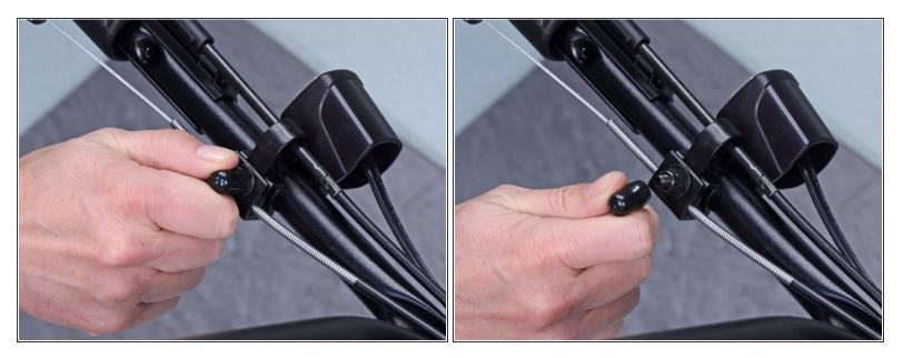
• Remove the black silicone cap covering the nut on the kill switch and upper cable guide assembly.
