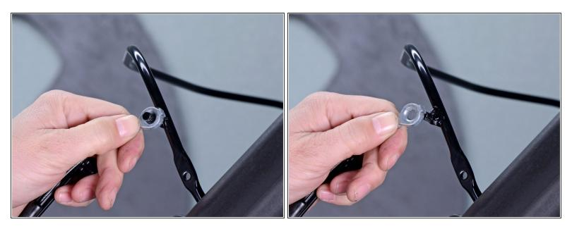
• Remove the brake cable from the brake handle.
