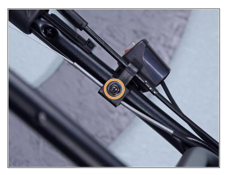
Use a 7/16 inch socket or wrench to remove the nut securing the kill switch and upper cable guide assembly.
