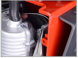
• Use a pair of needle nose pliers to unhook the traction cable spring from the transmission.
