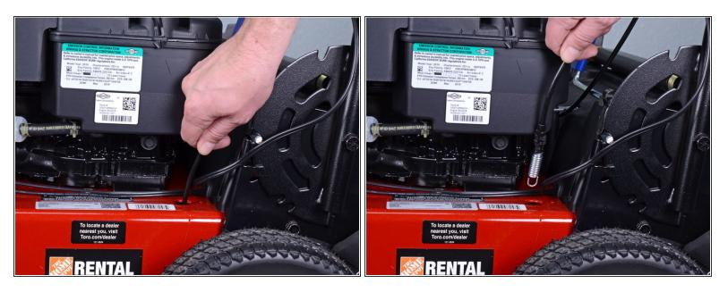
Pull the traction cable out through the cutout in the frame.
