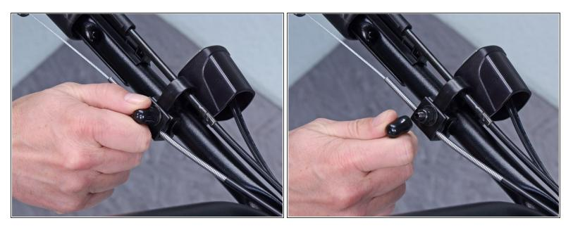
• Remove the black silicone cap covering the nut on the switch and upper cable guide assembly.
