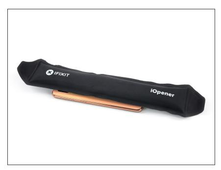
Apply a <u>heated iOpener</u> to the back cover to loosen the adhesive underneath. Apply the iOpener for at least two minutes.
