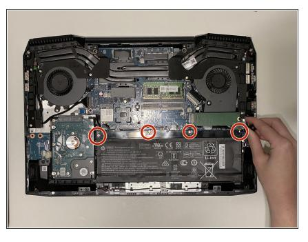
Remove the four 1.2 mm screws from the top of the battery using a Phillips #00 screwdriver.
