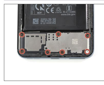
Use a Phillips #00 screwdriver to remove the seven 3.6 mmlong screws.
