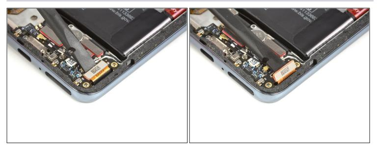
• Use the flat edge of a spudger to pry up and disconnect the display connector from its daughterboard socket.
