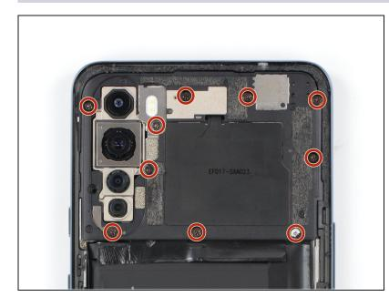
• Use a Phillips #00 screwdriver to remove the ten 3.6 mm-long screws from the motherboard cover.
