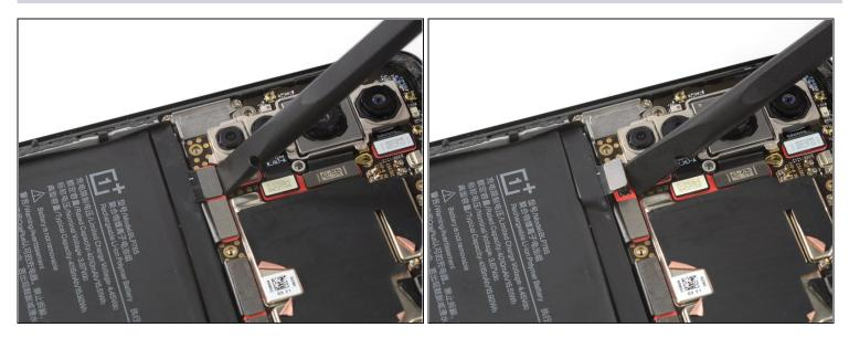
• Use a spudger to disconnect the battery by prying the connector straight up from its socket.
