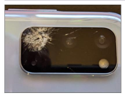
one complete. Note: The lens is held on with adhesive so we will need to heat the area. A blow dryer will work or a heat gun will get the job done. If you have a puncture you can use some tweezers to begin pulling up the glass there. Please NOTE, look at the next step photo to see where the lens resides.
