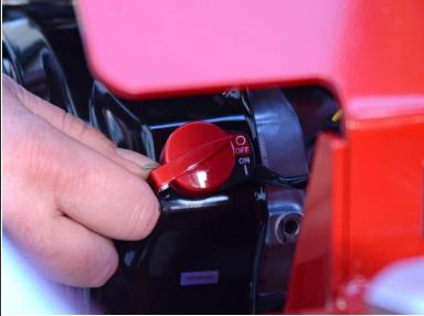
Flip the red engine ON/OFF switch to the OFF position.
