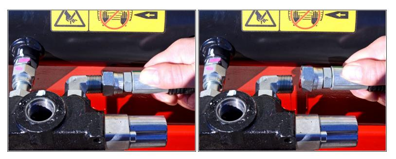
Remove the piston extension hose from the rear L-fitting.
