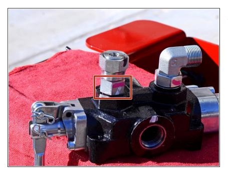
Use an adjustable wrench to loosen the nut securing the piston contraction fitting to the control valve.
