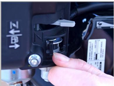
• Flip the fuel valve lever to the **OFF** position.
