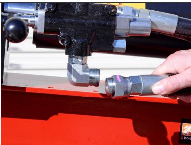
Remove the input hose from the bottom L-fitting.
