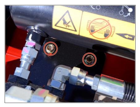
Use a 9/16 inch socket to remove the two bolts securing the control valve bracket to the frame.
