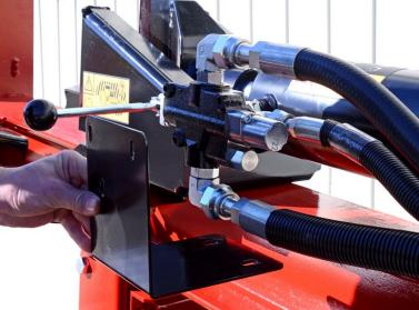
Remove the control valve bracket.
