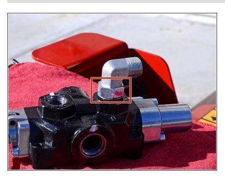
Use an adjustable wrench to loosen the nut securing the L-fitting to the rear of the control valve.
