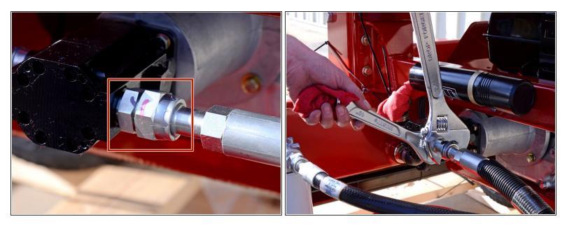
Use two adjustable wrenches to loosen the nut holding the input hose to the fitting on the right side of the pump.
