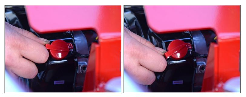
• Flip the red engine ON/OFF switch to the **OFF** position.
