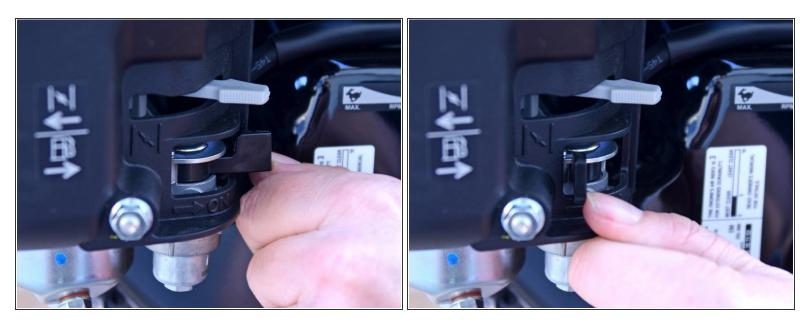
• Flip the fuel valve lever to the **OFF** position.
