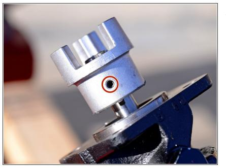
Use a 2.5 mm hex key to loosen the pump-side flex coupler's set screw until the flex coupler moves freely on the shaft.
