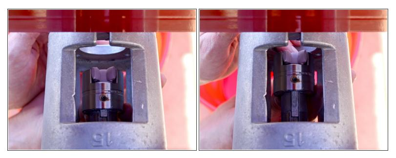
Reaching underneath the device, through the flex coupler housing access cutout, slide the motorside flex coupler off of the shaft.
