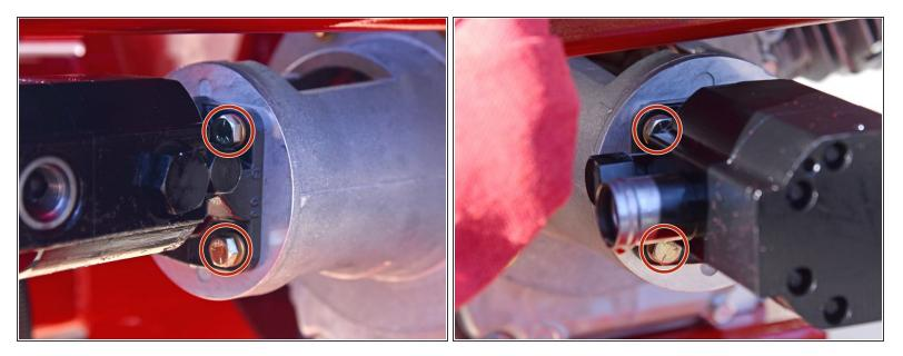
• Use a 1/2 inch wrench to remove the four bolts securing the pump to the flex coupler housing.
