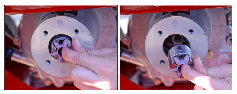
• Remove the motor-side flex coupler.
