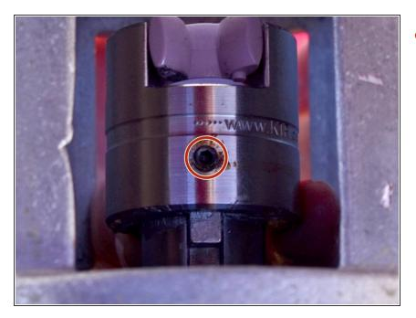
• Use a 2.5 mm hex key to remove the motor-side flex coupler's set screw.
