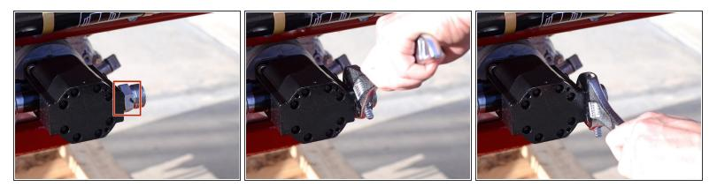
Use an adjustable wrench to remove the fitting on the right side of the pump.
