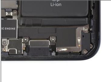
• Remove the four 1.5 mm-long Phillips #000 screws securing the speaker.
