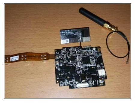
The main motherboard with antenna card, and the chance of upgrading it with a generic antenna, improving reception and transmission.
