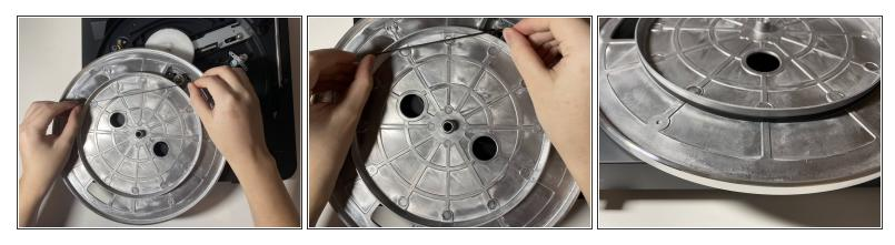
Place the new belt around the inner lap on the upside-down platter.
