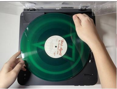
Open the top plastic cover and remove the record and rubber mat.
