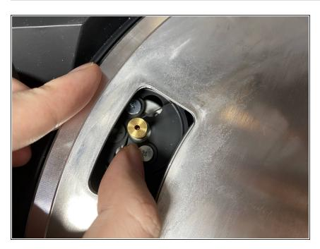
Put the belt around the motor pulley.
