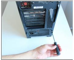
Using the Phillips #0 screwdriver, screw in the two 15 mm screws back into the case to lock the panel into place.
