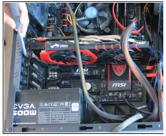
• Use the Phillips #0 to remove the three 14mm Phillips screws from the GPU and motherboard so we can remove the GPU later.
