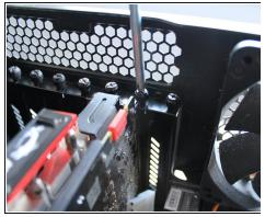
Screw the three 14 mm Phillips screws back in using the Phillips #0 screwdriver.
