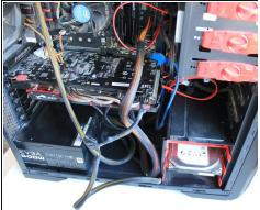
• Reconnect the 8-Pin Male Cable from the PSU into the GPU to power it when we turn it on.
