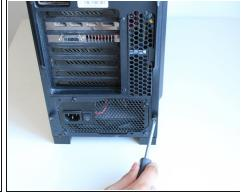
Use the Phillips #0 screwdriver to remove the two 15 mm screws on the glass panel side and remove the panel.
