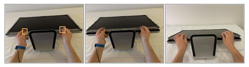
• Use the black tabs to raise the bottom edge of the LCD a few inches to access the cables inside.
