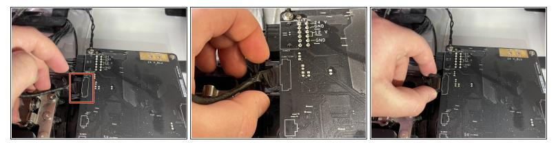
Squeeze the sides of the function cable connector on the top left edge of the logic board and pull it straight out.
