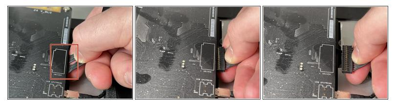
Pinch the LED backlight driver cable on the underside of the center right edge of the logic board and pull straight out.
