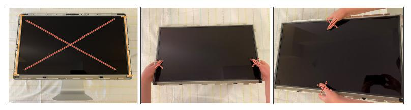
(i) First Steps Remove the glass panel as shown on step 2.
