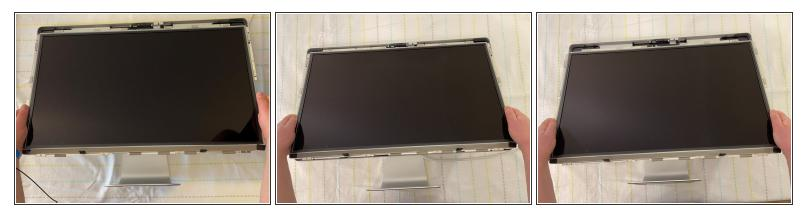
Handle the LCD panel by the edges and lift it upwards until it separates from the rest of the enclosure.
