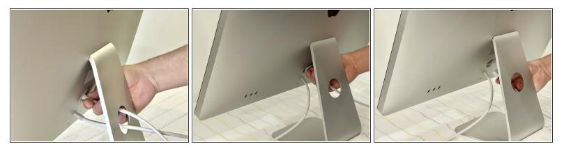
• Before beginning any work on your Mac: Unplug the computer and wait for 2 minutes in order for the power supply's capacitors to discharge.
