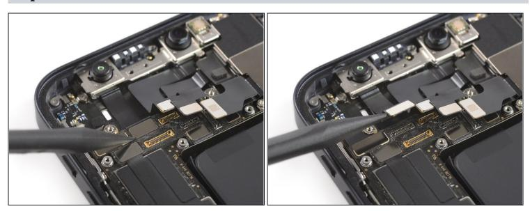
• Use a spudger to disconnect the infrared camera flex cable by prying it straight up from its socket.
