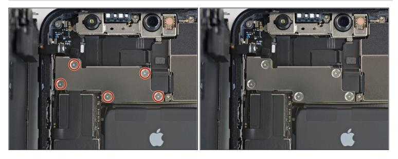
Remove the five 1 mm-long Y000 screws securing the front sensor assembly cover bracket.
