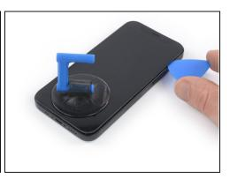
• Slide the opening pick around the bottom right corner and along the right edge of the iPhone, slicing through the adhesive holding the display in place.
