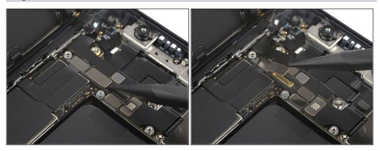
• Use a spudger or a clean fingernail to disconnect the front sensor assembly cable connector.
