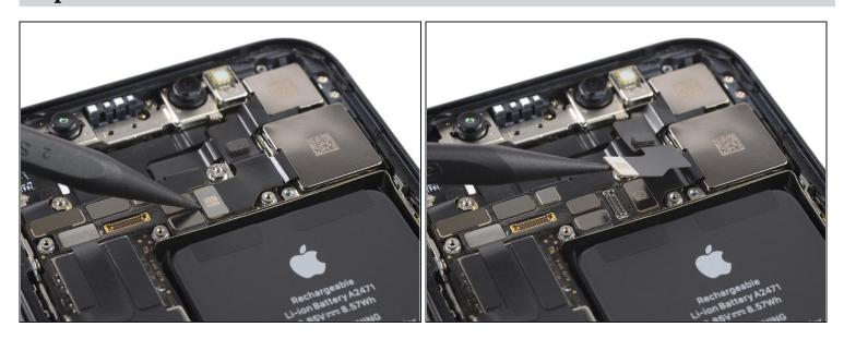
• Use a spudger to disconnect the ultra wide angle camera flex cable by prying it straight up from its socket.
