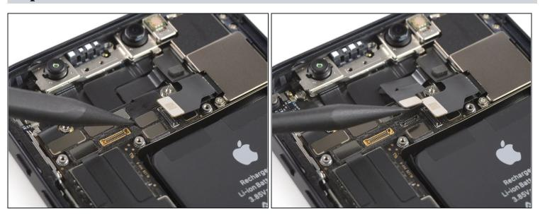
• Use a spudger to disconnect the dot projector flex cable by prying it straight up from its socket.
