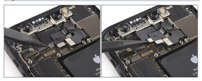
• Use a spudger to disconnect the selfie camera flex cable by prying it straight up from its socket.
