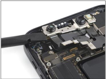
Use a spudger to pry up the front facing camera assembly.
