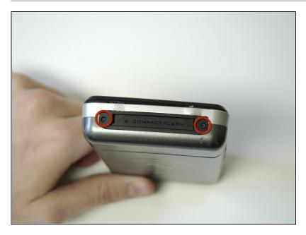
Remove the 2 screws (3.5 mm) on the Compact Flash insert, located on the left hand side, with a Phillips #000 screwdriver.
