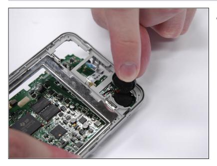
• Turn the speaker on its side so it can fit through the casing and the motherboard can be removed.
