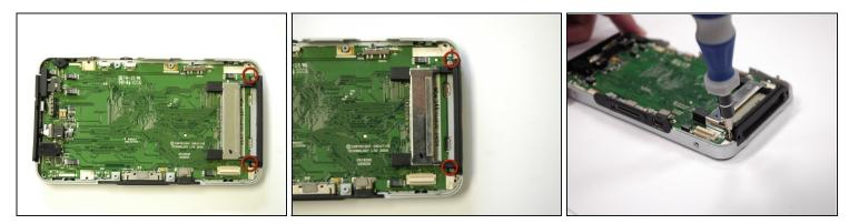
• Remove 2 screws (3.5 mm) on the black compact flash input using a Phillips #0.
