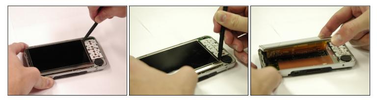
• Use a spudger to separate the metal tabs that hold the screen in place on the right side.
