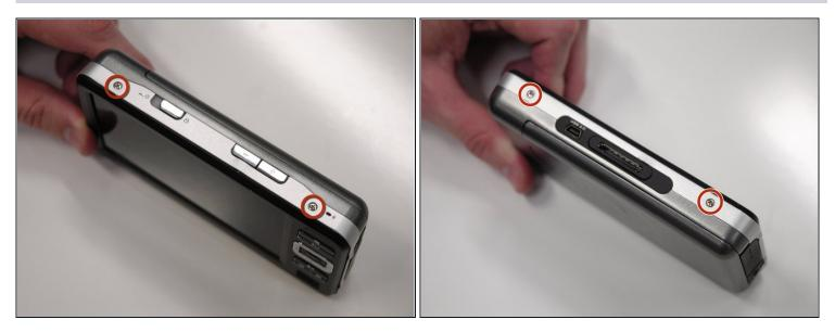
• Remove the two screws (2.5 mm) on the top and bottom of the device using a Phillips #0 screwdriver.
