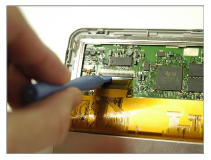
• Use a plastic opening tool to get underneath the black flap on the larger ribbon cable connection and lift it.
