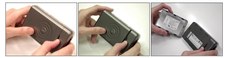
• Push the black button and slide the battery casing to the left simultaneously, until the battery is completely separated from the device.
