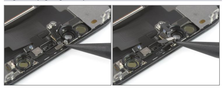
• Use the pointed end of a spudger to carefully pry the proximity sensor out of its recess.
