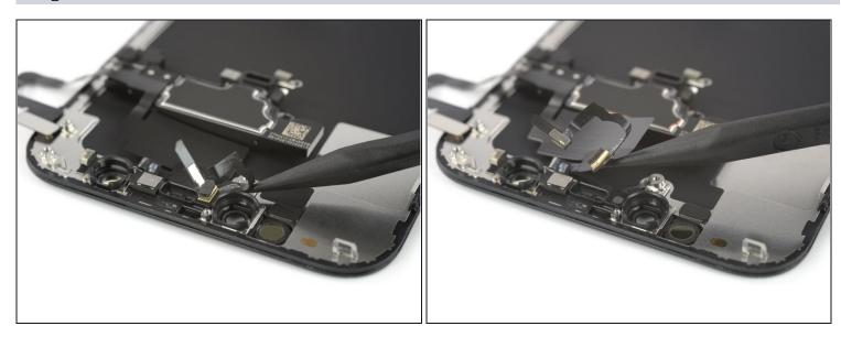
• Slide a spudger underneath the wide sensor assembly flex cable to separate it from the screen.
