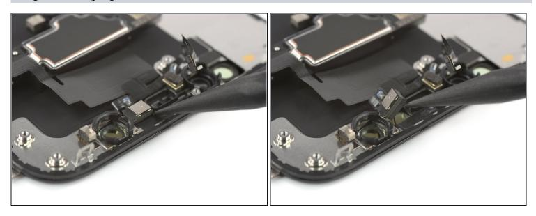
Use a spudger or a pair of tweezers to pry the flood illuminator out of its recess.
