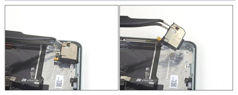
• Use tweezers to remove the loudspeaker from the rear case.
