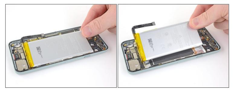
⚠ Do not reuse the battery if it has been deformed or damaged, as doing so is a potential safety hazard. Replace it with a new battery.
