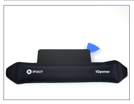
• Apply a heated iOpener to the left edge of the screen for one minute.
