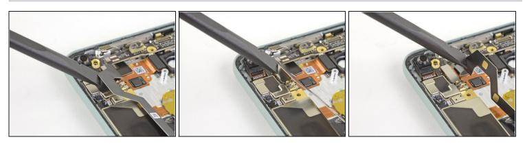
• Use a spudger to gently fold the flex cable covering the rear case press connector out of the way.
