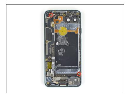
• Use a T3 Torx driver to remove the two 2.9 mm screws securing the motherboard to the rear case.
