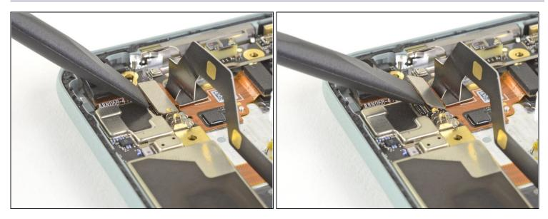
• Use the spudger to disconnect the rear case press connector.
