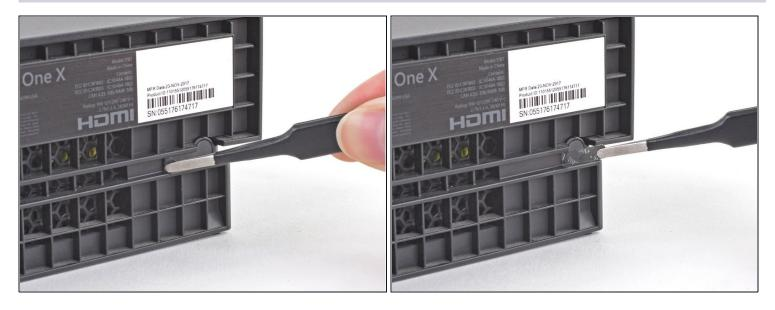
Use blunt tweezers to peel off the sticker covering the right-side screw on the back of the console.
