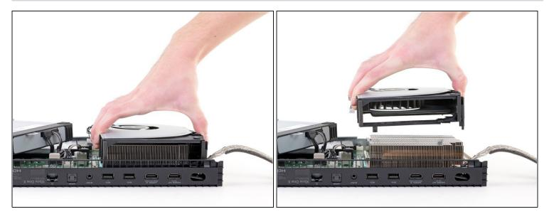
• Lift the fan case up to remove it from the console.
