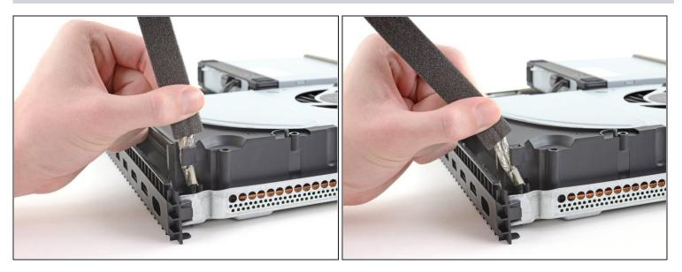
• While holding the power supply above the console, move the two grey cables out of the plastic hook on the fan case.
