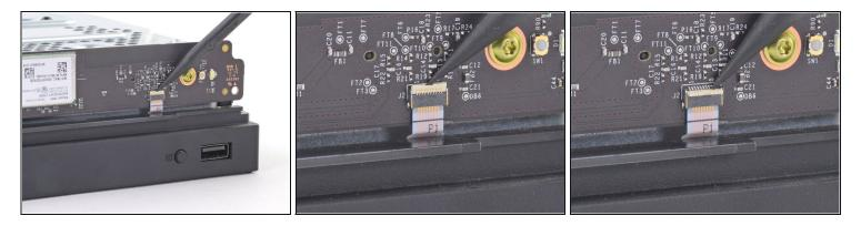
Use the pointed end of a spudger, an opening tool, or your fingernail to flip down the small, hinged locking flap on the ribbon cable <u>ZIF connector</u> on the front circuit board.
