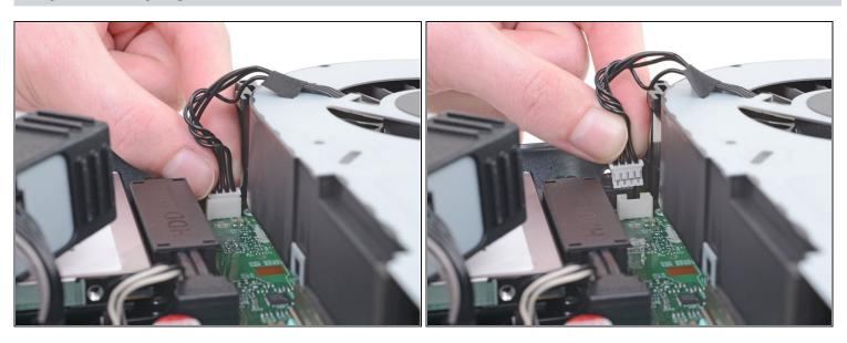
• Unplug the bundled cable connector connecting the fan to the motherboard by pulling directly upward.
