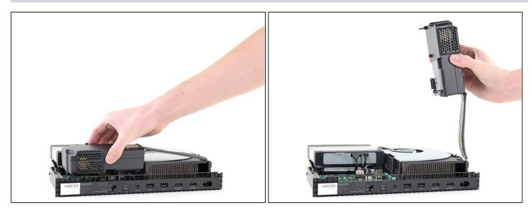
• Lift the power supply so that the cables are at a 90 degree angle.
