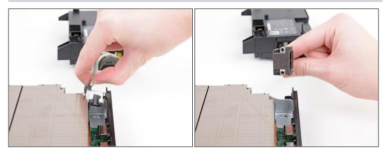
• Lift the power supply socket out of the upper metal case.
