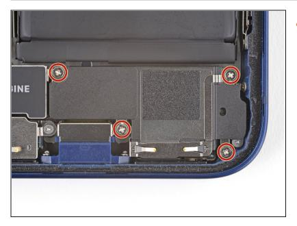
Use a Phillips driver to remove the four 1.6 mm screws securing the loudspeaker.
