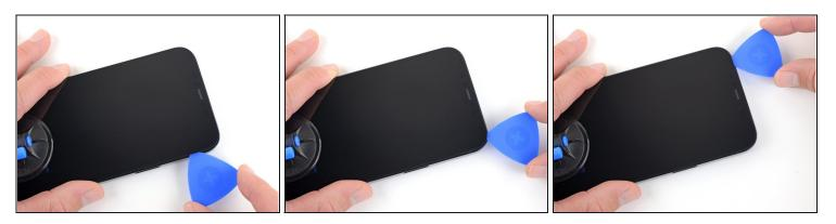
• Slide the opening pick around the top right corner of the iPhone to separate the top adhesive.
