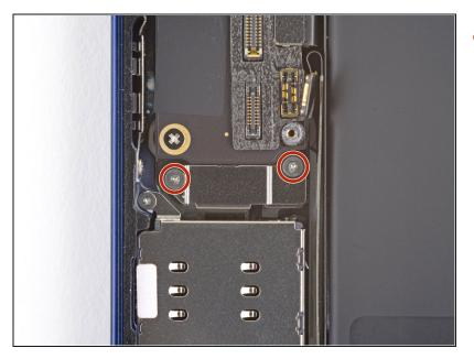
Use a Y000 driver to remove the two 1.4 mm long screws securing the SIM card reader connector cover.
