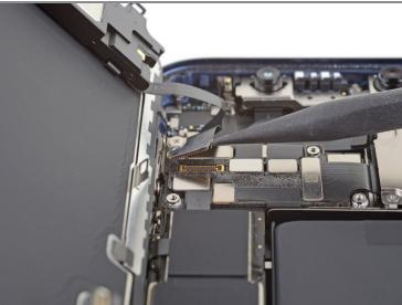
• Use a spudger or a fingernail to disconnect the front sensor assembly cable connector.
