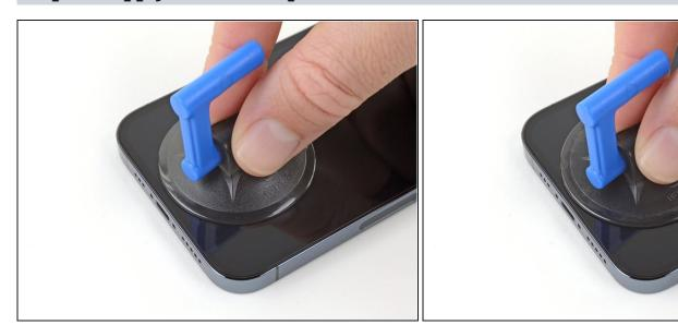
• If you're using a single suction handle, apply it to the bottom edge of the phone, while avoiding the very edge of the glass.
