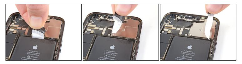
• Using the same procedure as before, pull the remaining two tabs, one at a time, to stretch and remove the remaining adhesive strip holding the battery in place. Try not to snag the adhesive on anything.
