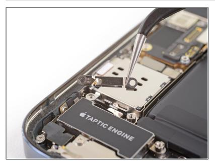
• Remove the Taptic Engine cable connector bracket.
