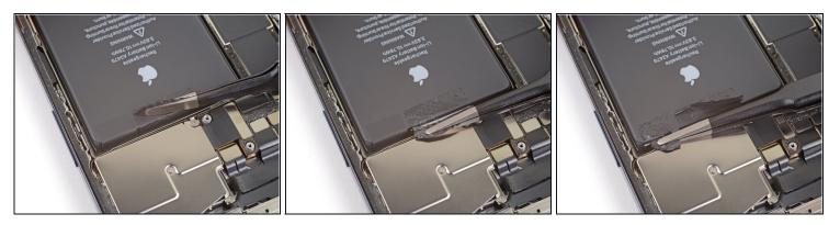
• Peel up the two remaining battery adhesive pull-tabs to un-stick them from the top edge of the battery.
