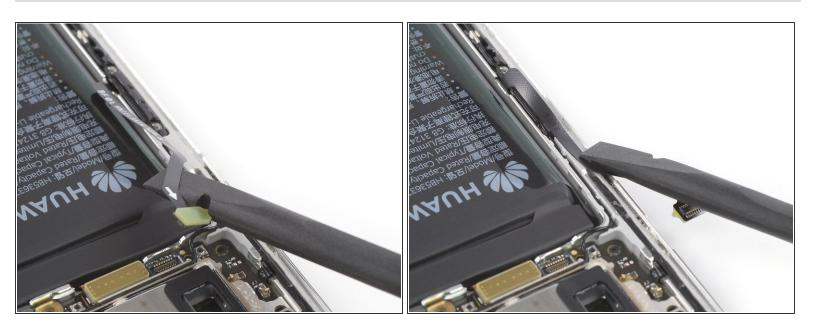
Fold the antenna cable to the side to avoid damaging it during the battery removal.
