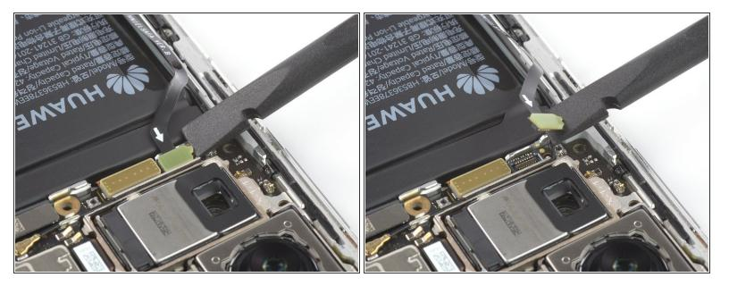
Use a spudger tor pry up and disconnect the antenna flex cable.
