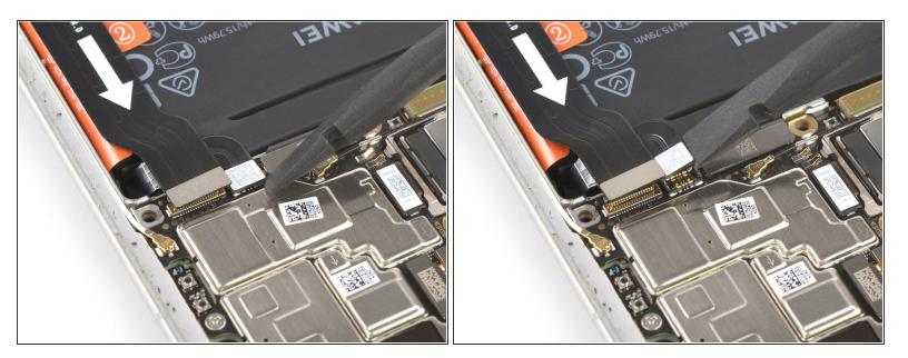
• Use the flat end of a spudger to pry up and disconnect the battery cable.
