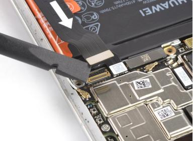
• Use the flat end of a spudger to pry up and disconnect the interconnect cable.
