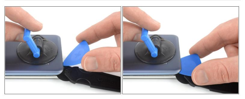
Insert an opening pick into the gap between rear glass and frame at the bottom left corner of your phone to prevent the adhesive from resealing.
