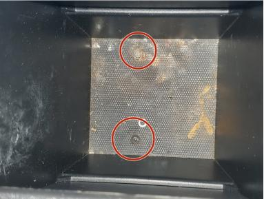
Unscrew the two 19mm screws within the storage compartment using the Phillips #1 screwdriver.
