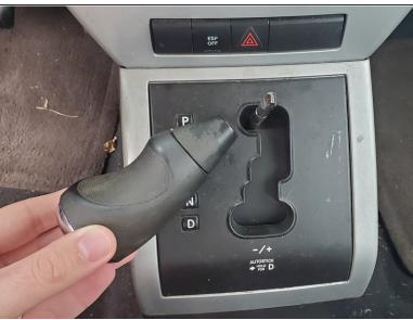
Remove the gear shifter handle, where it says PRDL (Park, Reverse, Neutral and Drive) next to it, by pulling it straight out in an upwards direction. It will take some force.
