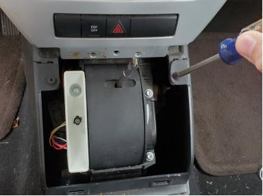
Remove the 19mm screws from the console using the Phillips #1 screwdriver.
