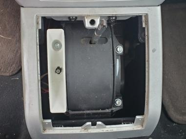
Remove the PRND bezel with a flat head screwdriver.
