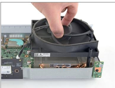
Lift the fan straight up to remove it from the motherboard.
