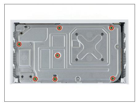
Use a T10 Torx driver to remove the seven 51 mm-long screws securing the chassis to the plastic case.
