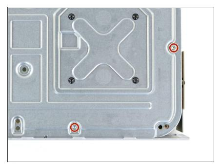
Use a T10 Torx driver to remove the two 11.3 mm-long screws securing the fan to the chassis.
