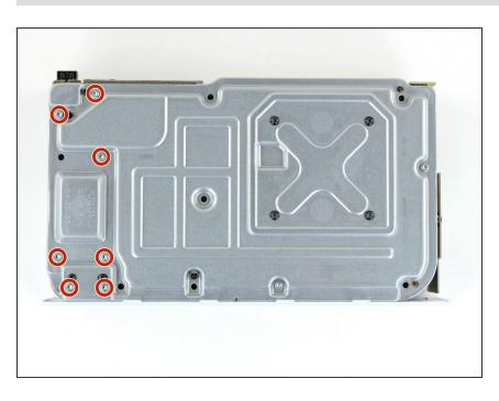
Use a T10 Torx driver to remove the seven 11.3 mm-long screws securing the power supply to the chassis.
