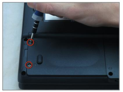
Loosen the two captive screws on the bottom left corner of the hard drive using a Phillips #1 screwdriver until you hear a click.
