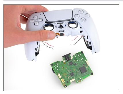
• Separate the controller from the motherboard.
