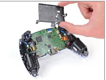
Lift the battery bracket out of the motherboard.
