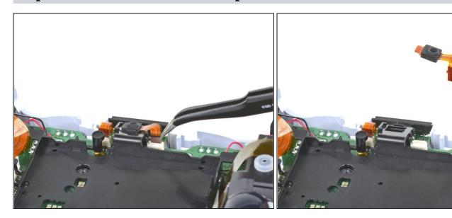
• Grab the lower microphone ribbon cable pull tab with your fingers or a pair of tweezers and disconnect it from the motherboard.
