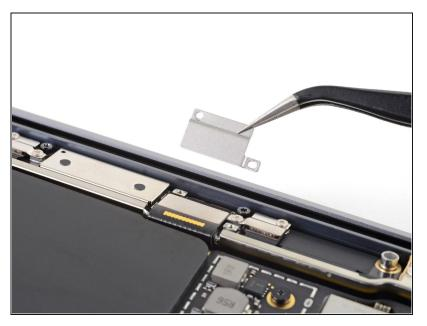
Remove the display cable connector cover.
