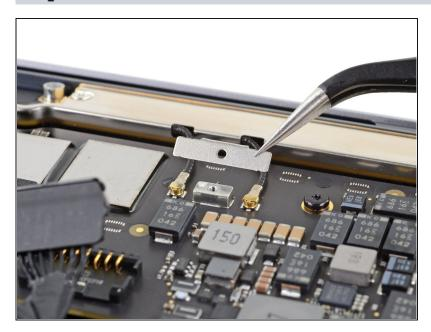
• Remove the antenna cable cover.
