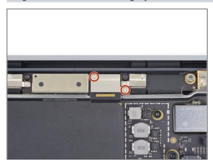
Use a T3 Torx driver to remove the two 1.5 mm screws securing the display cable connector cover.
