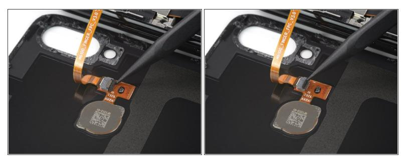
Use the pointed end of a spudger to open the ZIF connector by bringing its black flap in an upright position.
