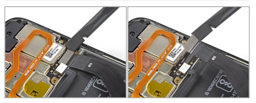
• Use the flat end of a spudger to pry up and disconnect the main flex cable.
