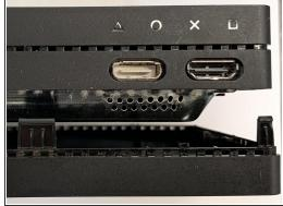
Use an opening tool to separate the bottom cover from the top.
