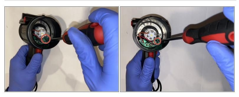
Using the JIS #00 screwdriver, remove the two screws securing the motherboard to the device.
