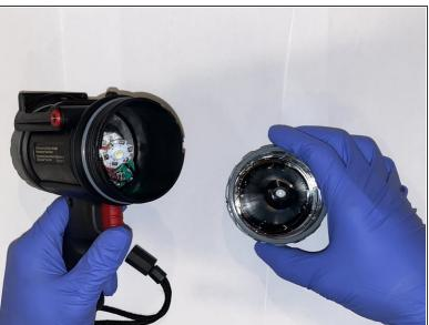
Twist the front cover of the spotlight in a counter-clockwise rotation and remove it from the device.
