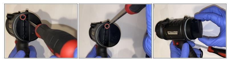
Using the JIS #00 screwdriver, remove the single screw securing the charging port and remove the charging port from the device.
