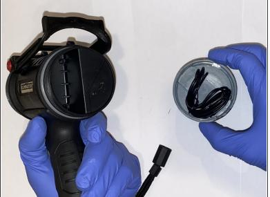
Remove the rear piece which is the protection cover for the charging port.
