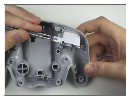
Once the spring is removed, take out the shoulder buttons by pulling down and out.
