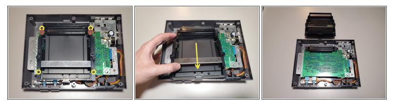
Remove four 13.25mm Phillips screws from the four corners of the cartridge tray. *Your system may only have two screws on the bottom*
