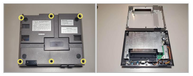
• Remove six **13.25mm Phillips screws** on the bottom of the system.
