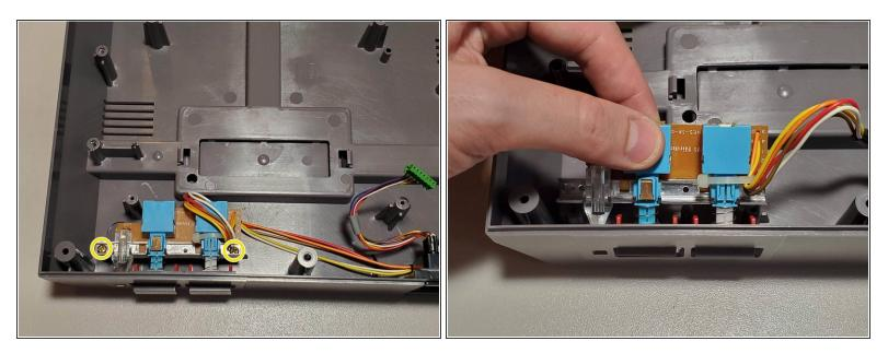
Remove two 13.25mm Phillips screws from the button assembly. Lift slightly in the back and then up and away from the housing to remove.
