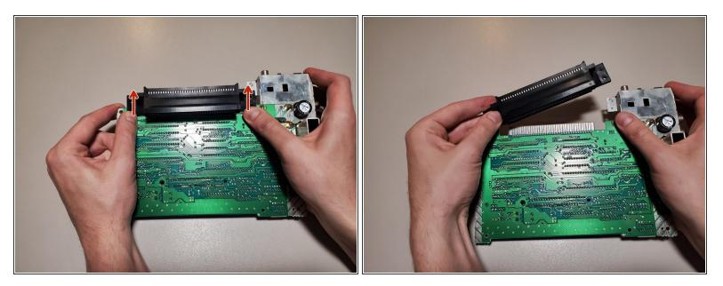
To remove the 72-Pin connector, apply force to each edge and slide the connector off the contacts on the motherboard.
