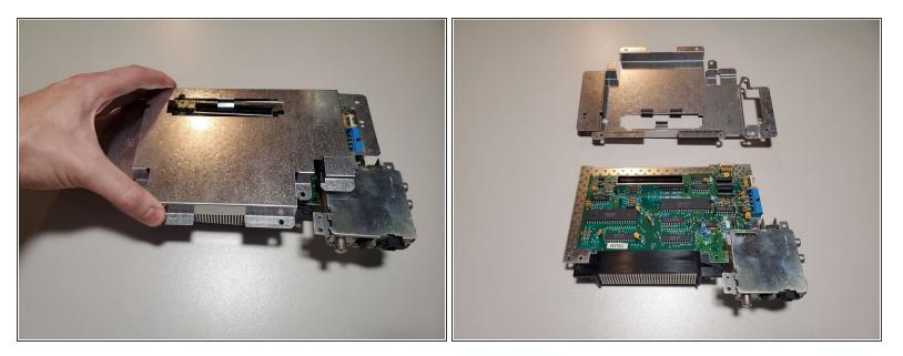
• The bottom RF shield is held on by tension around the expansion port. Lift the shield up and away from the motherboard.
