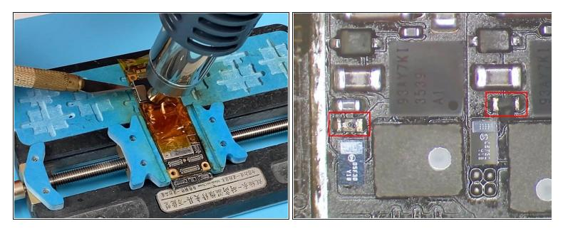
Heat the shielding cover with Hot Air Gun at 380 °C and airflow 60. Pry up the shielding cover with a Sculpture Knife. It can be seen under the microscope that R5651 and R5661 are burnt out.
