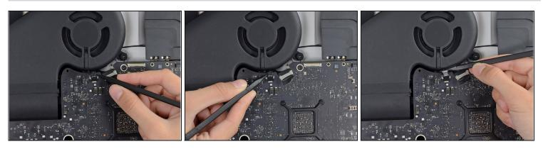
• Use the tip of a spudger to disconnect the fan cable's connector from its socket on the logic board.
