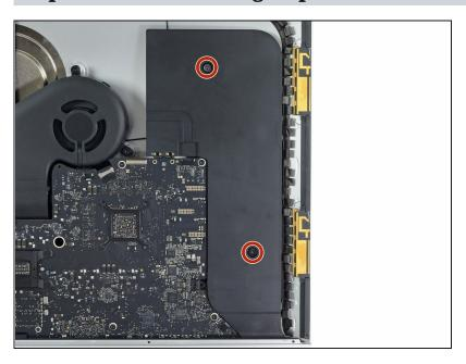
• Remove two 9.8 mm T8 screws.
