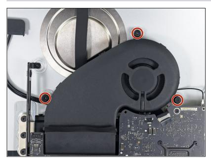
• Remove three 12.4 mm T10 screws securing the fan to the rear case.
