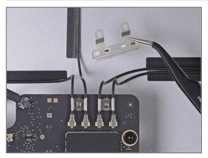
Remove the metal bracket securing the antenna cables to the logic board.
