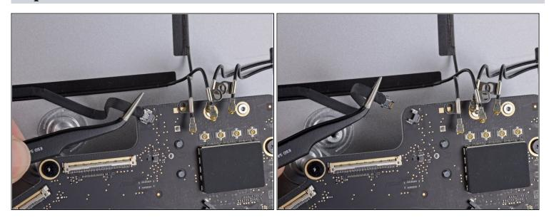
• Use a pair of tweezers or your fingers to disconnect the ribbon cable left of the antenna cables from the logic board.
