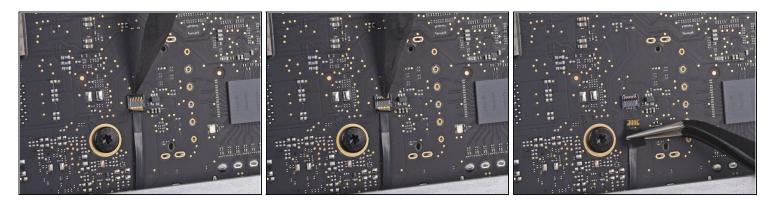
• Use the tip of a spudger to flip open the retaining flap on the microphone ribbon cable <u>ZIF socket</u>.
