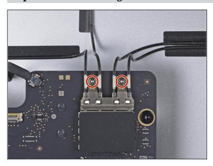
Use a T5 Torx screwdriver to remove the two 4 mm screws securing the AirPort/Bluetooth antenna cables.
