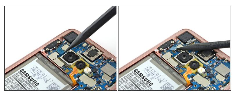
Use the point of a spudger to pry up and disconnect the fingerprint sensor connector from its motherboard socket.
