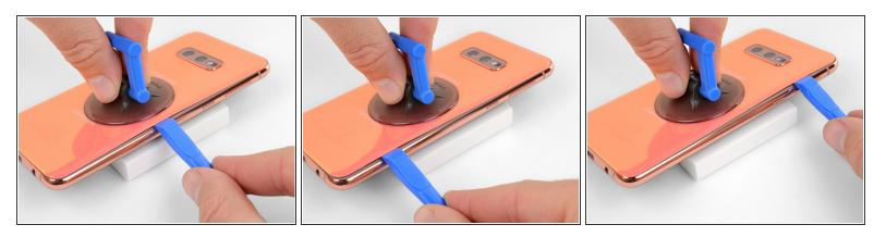
Slide the opening tool along the right edge of the phone to slice through the adhesive securing the back cover.
