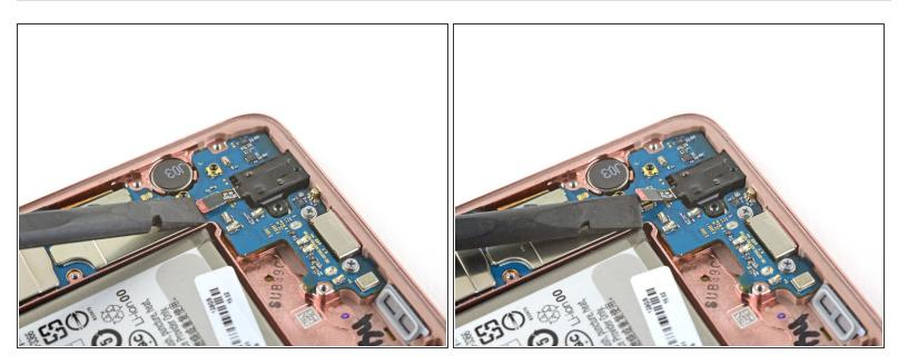
Use a spudger to pry up and disconnect the headphone jack connector from its motherboard socket.
