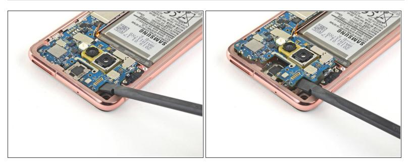
Use the flat end of a spudger to pry up and loosen the top portion of the motherboard.
