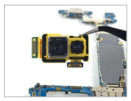
Remove the dual rear camera module.
