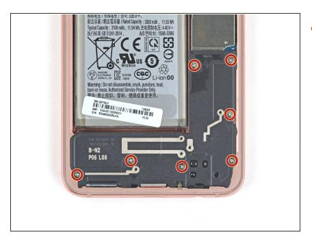
Use a Phillips driver to remove the seven 3.9 mm screws securing the loudspeaker.
