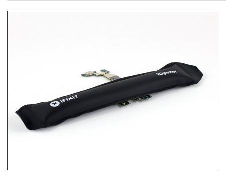
Apply a heated iOpener to the camera module for one minute to loosen the adhesive.
