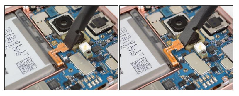
Use the flat end of a spudger to pry the battery connector straight up from its socket and disconnect it.
