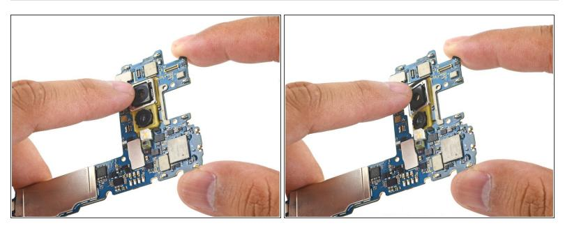
Use your finger to apply firm, steady pressure to the camera module to loosen it from the motherboard.
