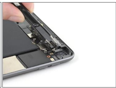
• Use a pair of tweezers to remove the power button bracket.
