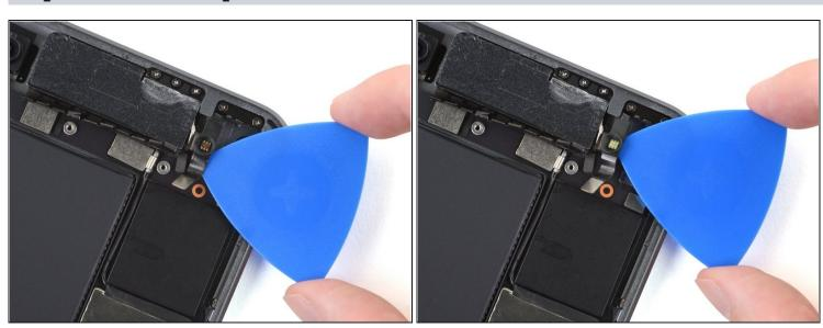
• Use an opening pick cut through the adhesive under the power button cable and detach it from the shelf.
