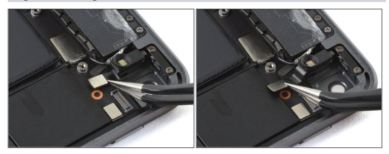
• Use a pair of <u>tweezers</u> to pull the power button cable out from under the shelf.
