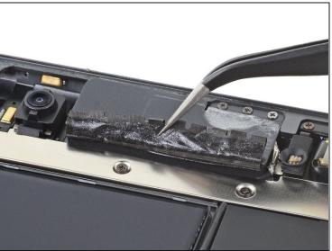
• Use a pair of <u>tweezers</u> to lift up the tape covering the press connector cover screws.
