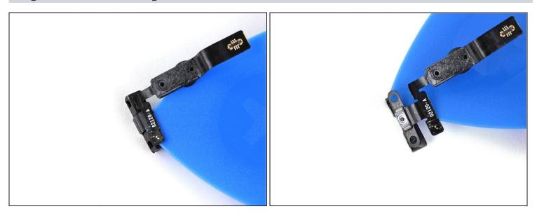
• Use an opening pick to cut through the adhesive securing the power button cable to the bracket.
