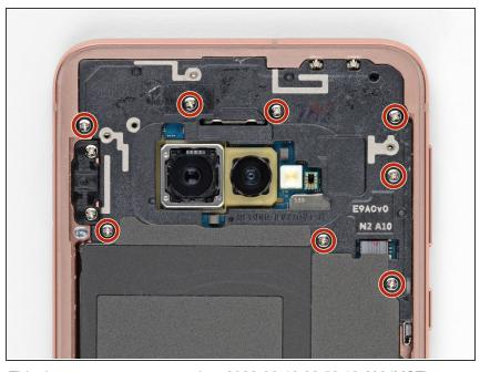
Remove the eight 3.9 mm Phillips screws securing the upper midframe to the phone.
