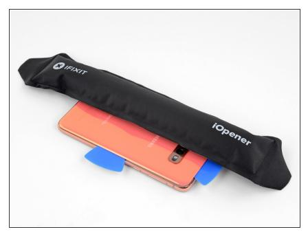
Apply a heated iOpener to the left edge of the phone for two minutes.
