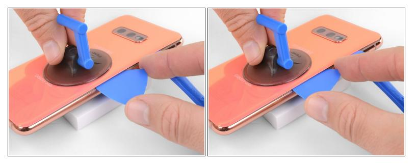
Insert an opening pick into the edge next to the opening tool. Leave the pick here to prevent the separated glue from re-adhering.
