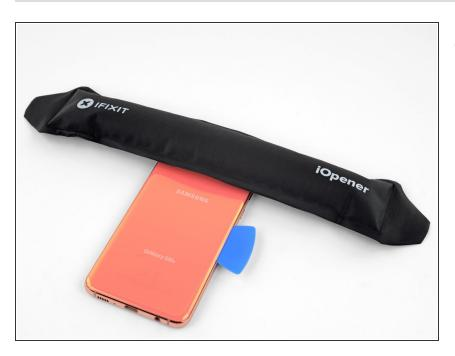
Apply a heated iOpener to the top edge of the phone for two minutes.
