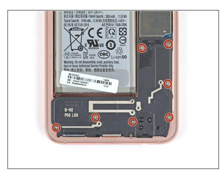
Use a Phillips driver to remove the seven 3.9 mm screws securing the loudspeaker.
