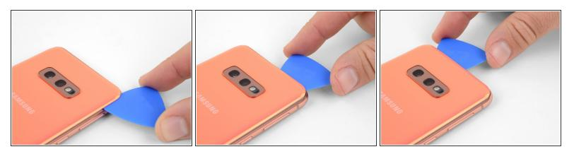
Insert an opening pick near the top right corner of the phone and slide it around the corner and across the top edge of the phone.
