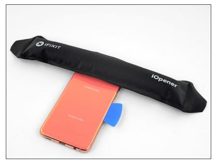
• Apply a heated iOpener to the top edge of the phone for two minutes.
