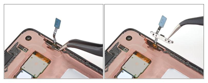
• Use a pair of tweezers to lift and remove the power button support bracket from its recess.
