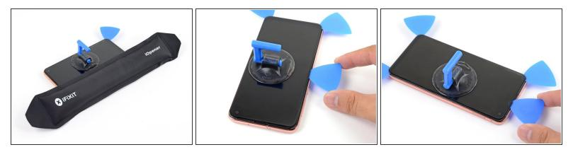
• Repeat the heating and slicing procedure for the remaining display sides.
