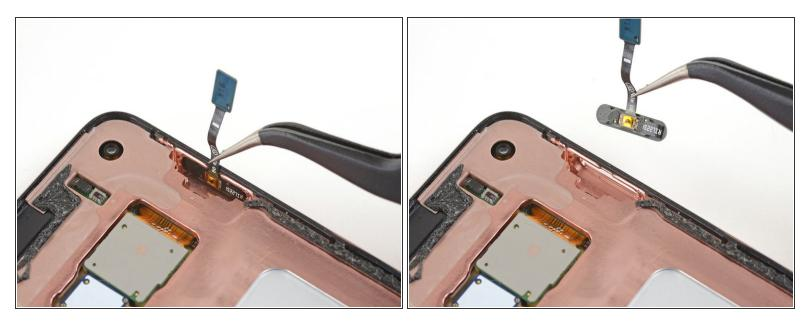
• Remove the fingerprint sensor from its recess.
