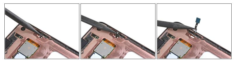
• Use the point of a spudger to gently pull the fingerprint sensor cable through its frame cutout.
