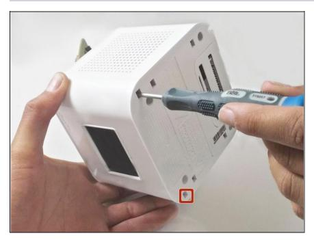
Insert a Phillips #1 screwdriver into the corner, square, holes and push the backlight board up away from the plastic casing.
