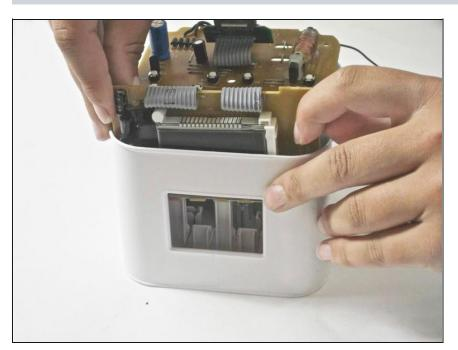
Carefully, pull up on the board to remove it entirely from the plastic casing.
