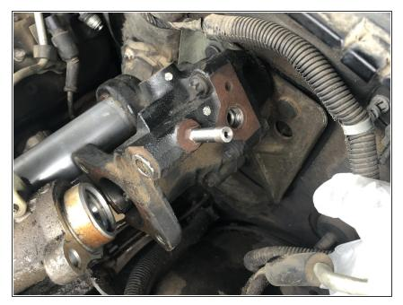
Once Hydroboost is in securely, attach Mounting plate between Hydroboost and Brake System.
