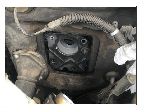
Once everything inside and out is free, pull the Hydroboost out revealing the hole in the firewall.
