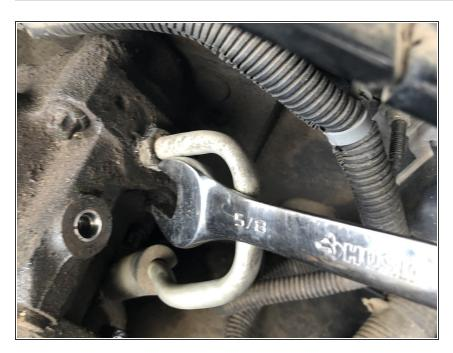
Use a 5/8" wrench to pull last feeder tube for power steering. Again be cautious of dirt and debris.
