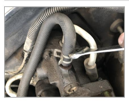
Use a pair of pliers or clamps to pull one of the power steering tubes off.
