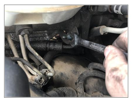
Use a box wrench or crescent wrench to take the two nuts off that connect the Hydroboost (against the firewall) to the brake system.
