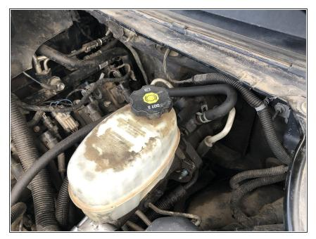
Open the hood, locate the brake fluid reservoir. Right under that is the Hydroboost device.
