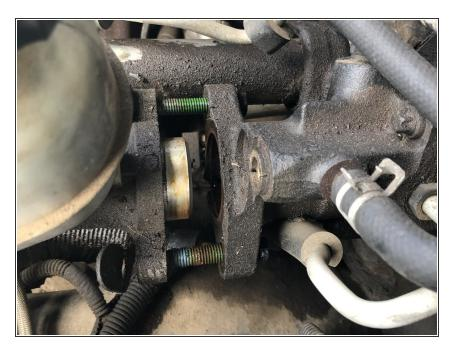
Everything should be free, so pull brake system away. Be careful not to put pressure on brake lines as they can break. Keep debris away from this too.
