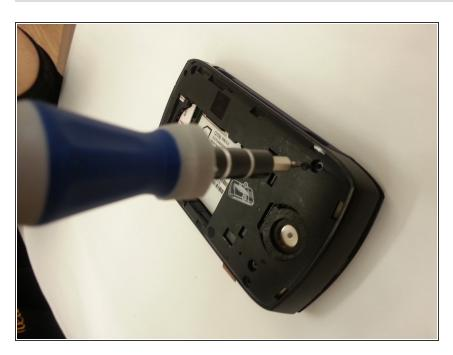
replace with new camera piece into casing and reassemble by reversing dissemble procedure
