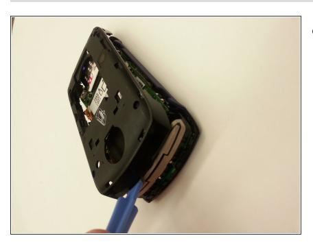
Remove camera piece from casing
